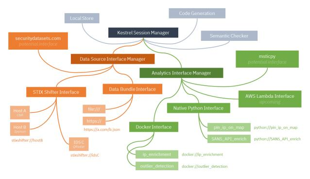
Illustrated in the figure above, Kestrel uses a two-level abstraction for both data source and analytics: (i) a data source or analytics *interface* defines how a data source or analytics executes, i.e., input, output, plus execution mechanism, and (ii) each data source or analytics is developed to be executed under one or more interfaces.
