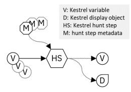
A command takes in one or more variables and maybe some metadata, for example, the path of a data source, the attributes to display, or the arguments to analytics. In general, the command can either yield nothing, a variable, a display object, or both a variable and a display object.
